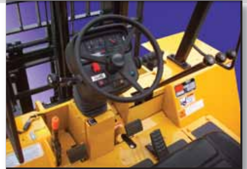
Steer Column : Self contained, fully adjustable, tilt and telescopic steer column
